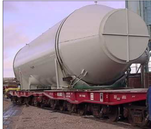
This 340 ton vessel was transported on two railcars as a bolstered load from Wyoming to Louisiana.
